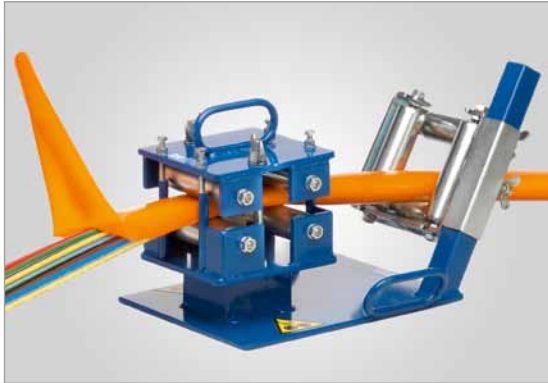
Cutting unit for bundles (equipment manufacturer Vetter, Lottstetten, Germany)
