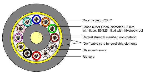
Principle drawing Example: A-DQ(BN)H 12x12 E9/125 0.36F3.5 + 0.22H18 LG
