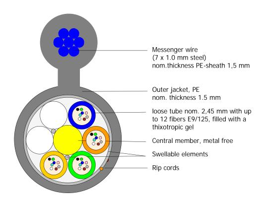
Principle drawing for a A-DT2Y 4x8 E9/125 0,36F3,5 + 0,22H18 LG (7x1,0)
