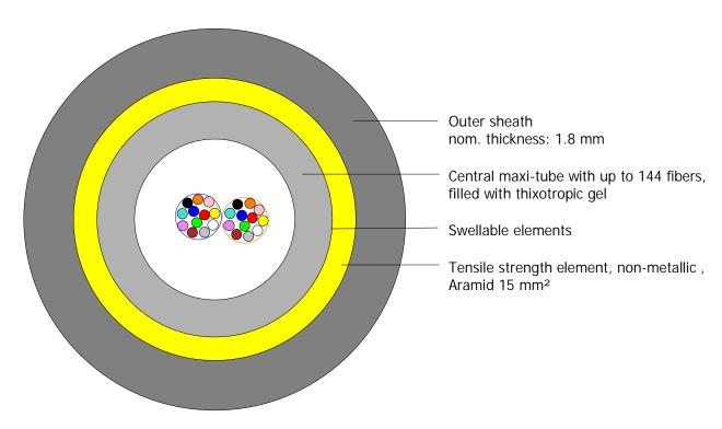
Principle drawing for a A-D(T)2Y 15 mm<sup>2</sup> 1x(2x12) E9/125 0.36F3.5 + 0.22H18
