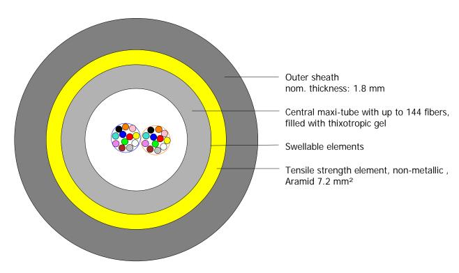
Principle drawing for a A A-D(T)2Y 7.2 mm<sup>2</sup> 1x(2x12) E9/125 0.36F3.5 + 0.22H18
